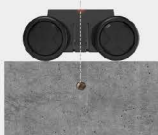
Accurately determinethe position of the rebar
